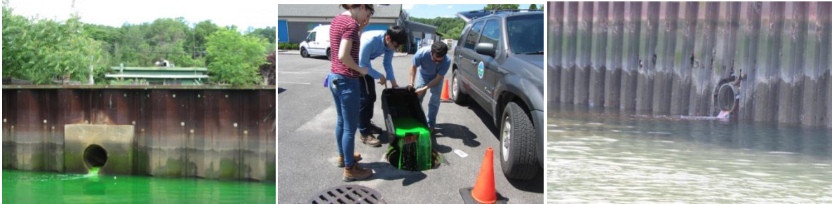
Dye testing to identify sources of discharges in Glen Cove Creek (photos by Carol DiPaolo, 6/7, 6/13, 11/28/17, (l-r))
