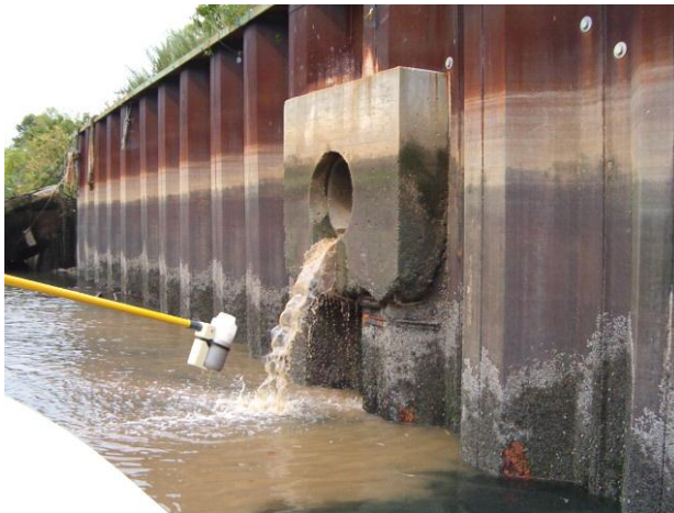
Sampling an unusual discharge from north side of Glen Cove Creek (photo by Carol Di Paolo)
